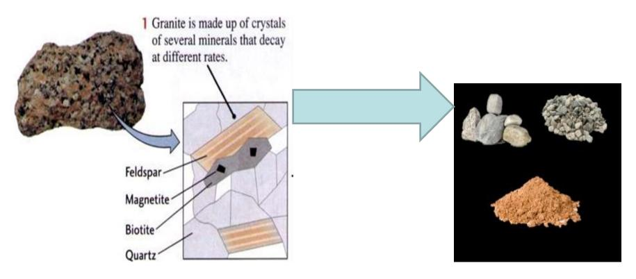
The minerals that make up rocks have different coefficients of linear and volumetric expansion, that is, they react differently to heating and cooling. These processes are especially active in areas with a continental climate, where there is a sharp difference in seasonal and daily temperatures.
